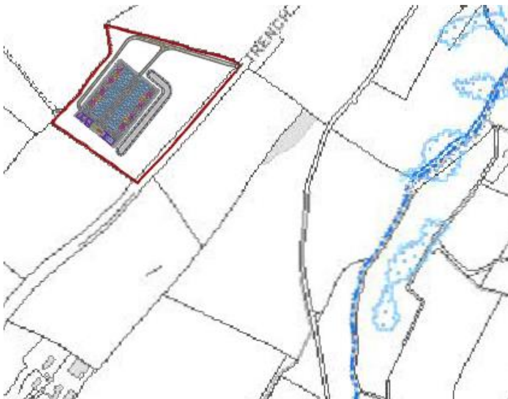
Figure 3 - Excerpt from DfI Rivers fluvial flood risk map, with proposed site boundary overlaid.
