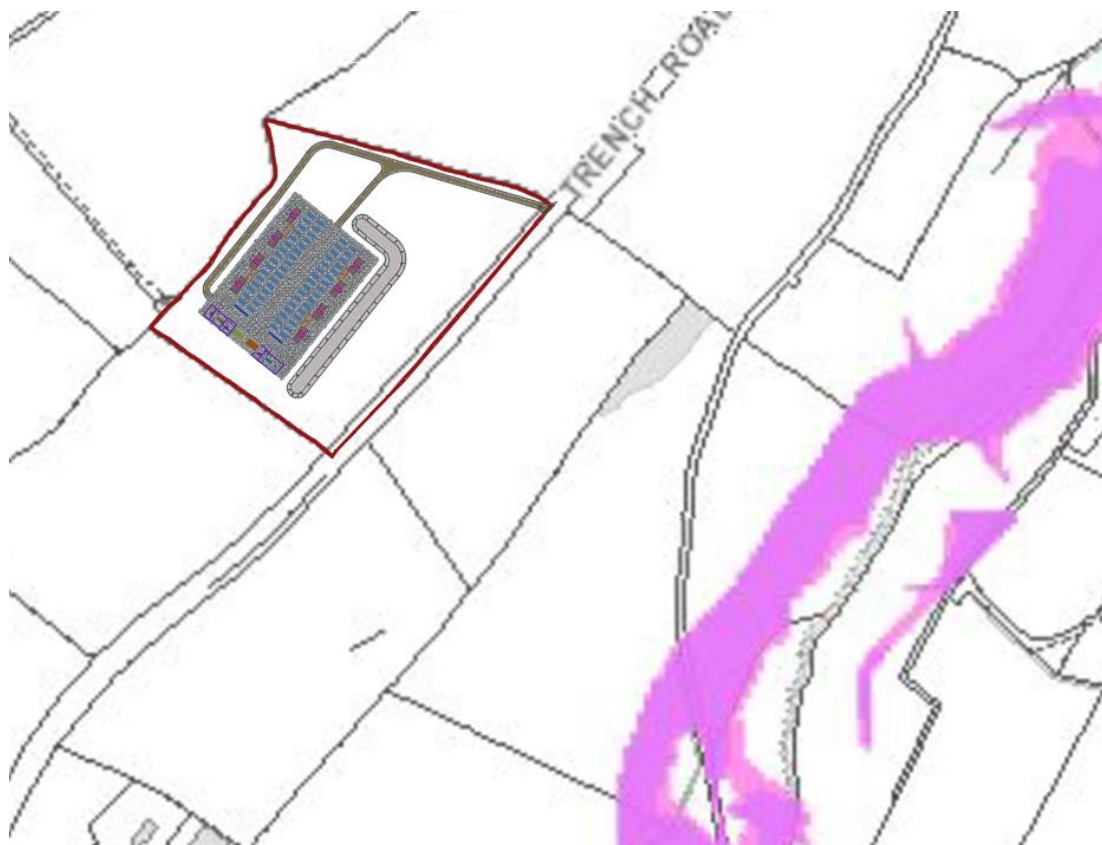
Figure 4 - Excerpt from DfI Rivers surface water flood risk map, with proposed site boundary overlaid.
